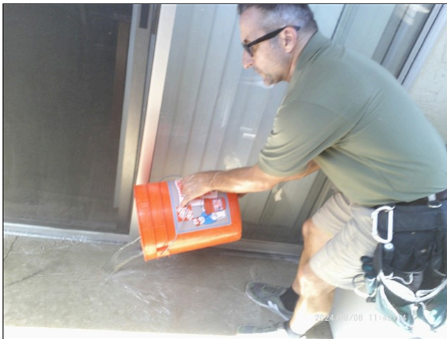
9.1 Inspector placing water on the walking surface to observe waterproofing and drainage performance.
