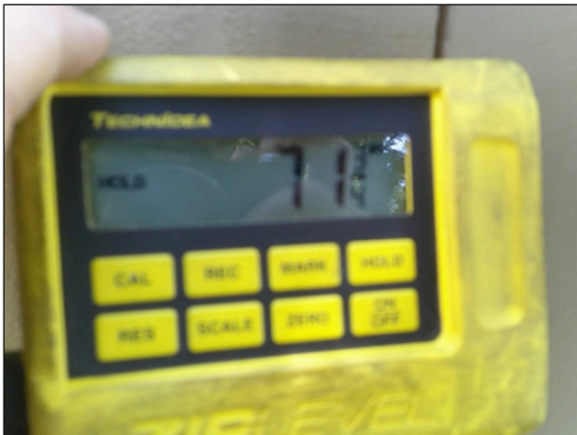
10.0 Precise vertical measurement between the "reference point" and "measured to" location.
